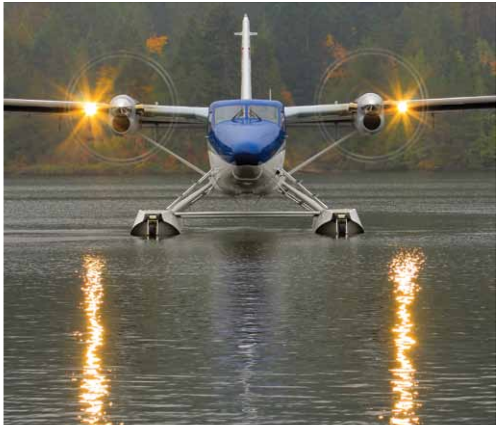
With six different landing-gear options, the Twin Otter 400 can operate from any land, water or polar environment.
