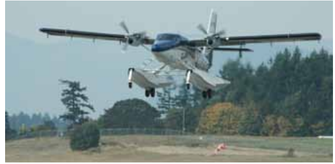
The Twin Otter 400 retains all the operational capability of its predecessors, enhanced by new PT-6A-34 engines.
